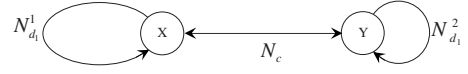
FIG. 13. A schematic of two mutually coupled nonidentical units with single self-feedback and single mutual coupling. N_{d_1}^1 and N_{d_1}^2 are the self-feedback delays of unit X and Y, respectively. N_c is the mutual delay.
